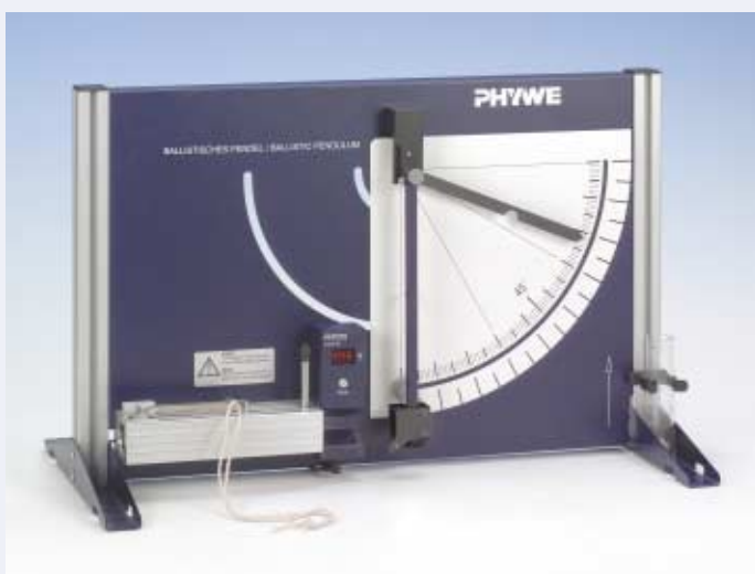
Experimental set-up with supplement for direct measurement of the initial velocity of the ball.
