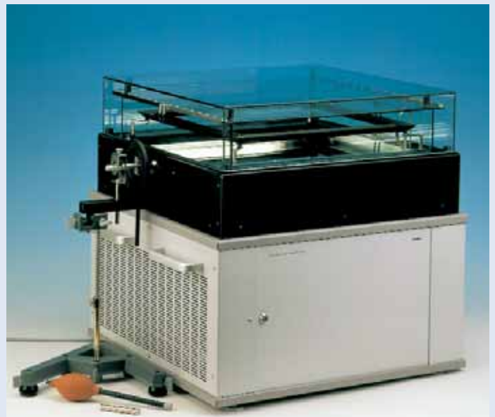
Experimental set-up: deflection of \beta -particles.
