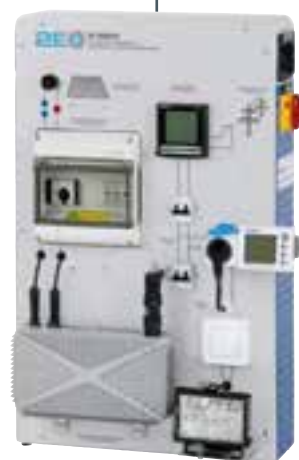
ET 250.01 Photovoltaic in grid-connected operation
