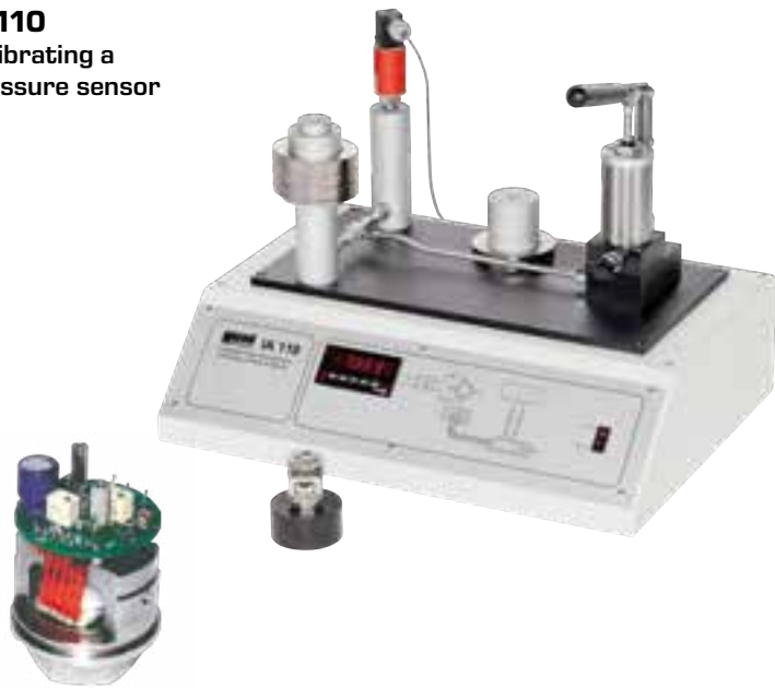
Interior layout of an electronic pressure sensor
