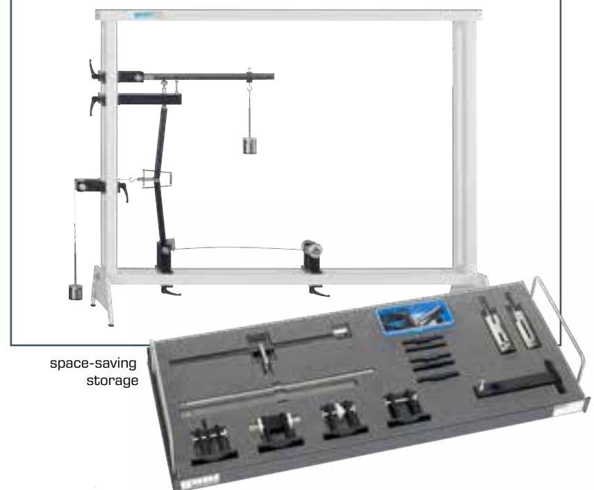
SE 110.19 Investigation of simple stability problems
