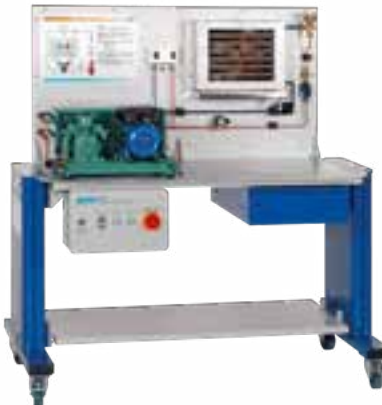
ET 192 Replacement of refrigeration components
