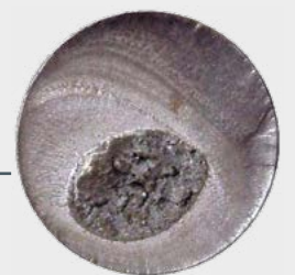
Analysis of the fracture surface following the fatigue strength test
