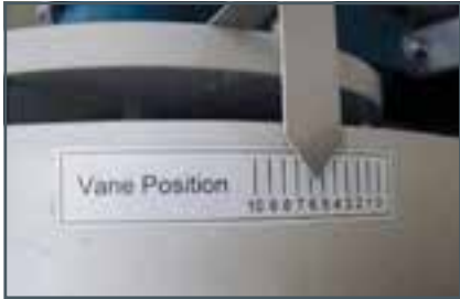
Position of the guide vanes in the Francis turbine
