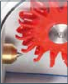
Needle nozzle and impeller of the Pelton turbine
