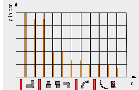
Sample measurement of the pressures between the various pipe elements
