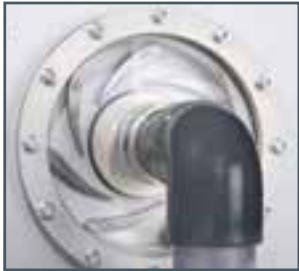
Vanes and impeller of the Francis turbine
