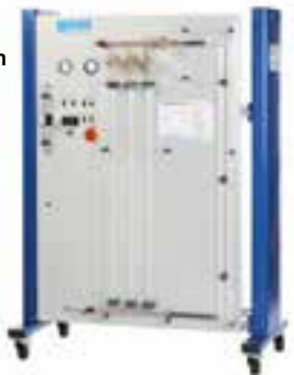
ET 460 Oil return in refrigeration systems
