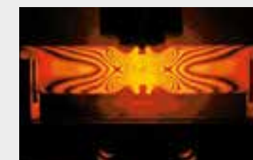
Model of a notched bar (FL 200.05) in monochromatic light
