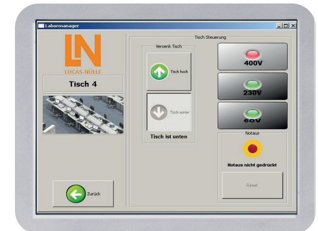
Control of individual stations
