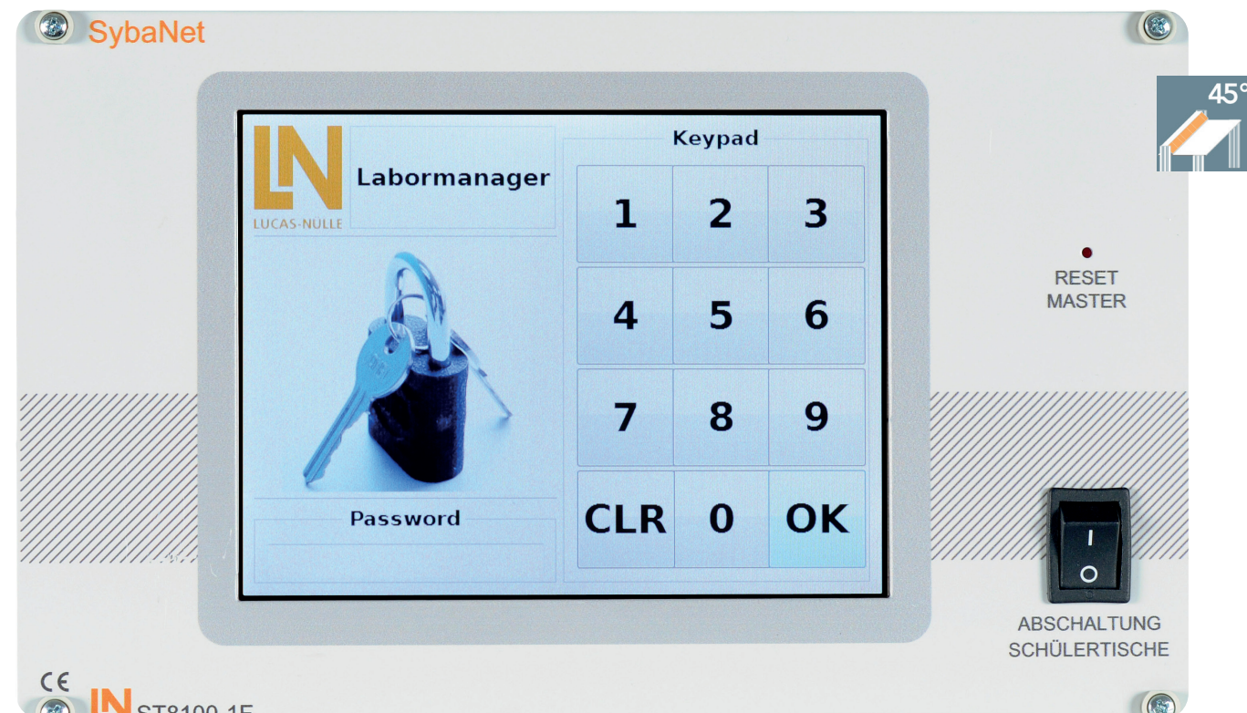
Lab manager with touch-panel PC, Art. No. ST8100-1E
