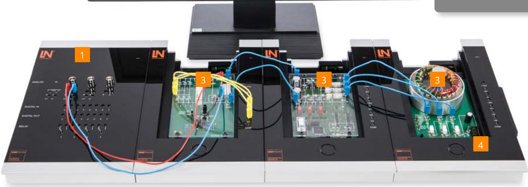
1 UniTrain-Interface Measurement and control interface: Analog/digital measurement inputs and voltage sources for the experiments.
